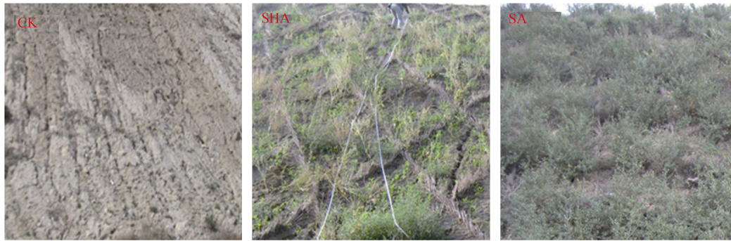
注：CK、SHA、SA 分别表示裸坡、沙柳方格+沙棘+沙打旺边坡、沙柳方格+沙打旺边坡 Note: CK, SHA and SA represent Bare slope, Vegetation slope with Salix cheilophila , Hippophaerhamnoides Linn. and Astragalus adsurgens Pall slope and Vegetation slope with Salix heilophila and Astragalus adsurgens Pall slope respectively.
