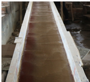
a. 含沙水流的波流耦合现象 a. Wave and current coupling phenomena in sand-laden flow b. 波流耦合中的波峰波谷状态 b. Wave crest and trough in wave-current coupling c. 含沙水流正常输沙现象 c. Normal sediment transport in sand-laden flow
