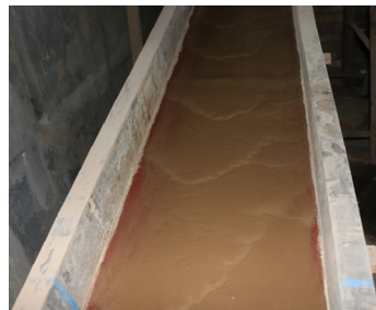
a. 含沙水流的波流耦合现象 a. Wave and current coupling phenomena in sand-laden flow b. 波流耦合中的波峰波谷状态 b. Wave crest and trough in wave-current coupling c. 含沙水流正常输沙现象 c. Normal sediment transport in sand-laden flow
