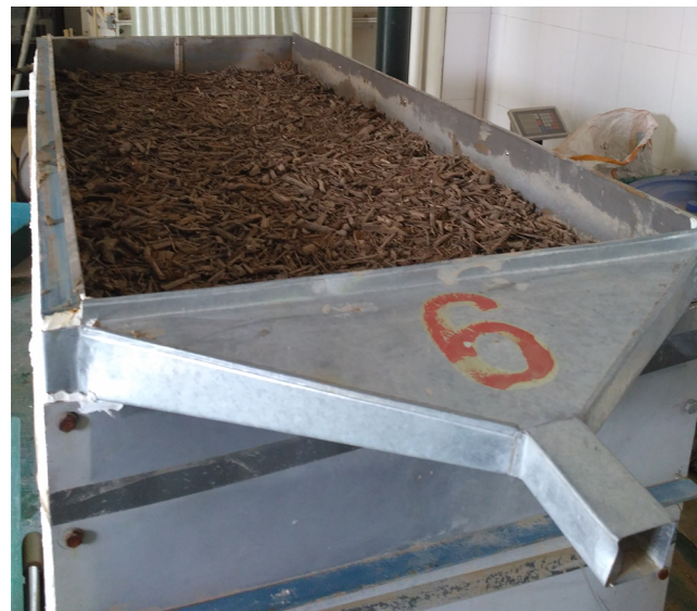
Fig. 1. Photograph of an experimental plot with mulching application rate at 1.48 \text{ kg m}^{-2} .
