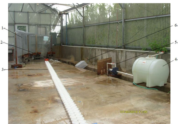
Figure 1. The indoor experimental setup: 1) screen, 2) sprinkler, 3) catch can, 4) tank, 5) pump, 6) flow meter.
