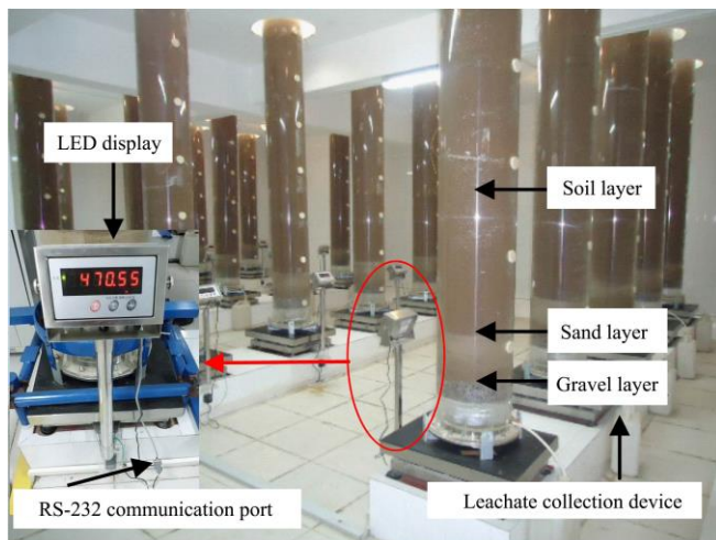
Figure 7 Underground portion of the root system monitoring system
