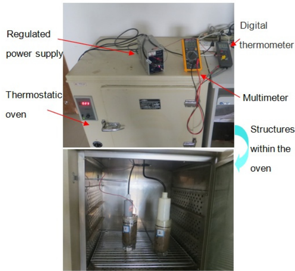
Figure 3. Pictures of the experimental system for measuring the output of the DSW-T2 and TM-100Y soil sensors.
