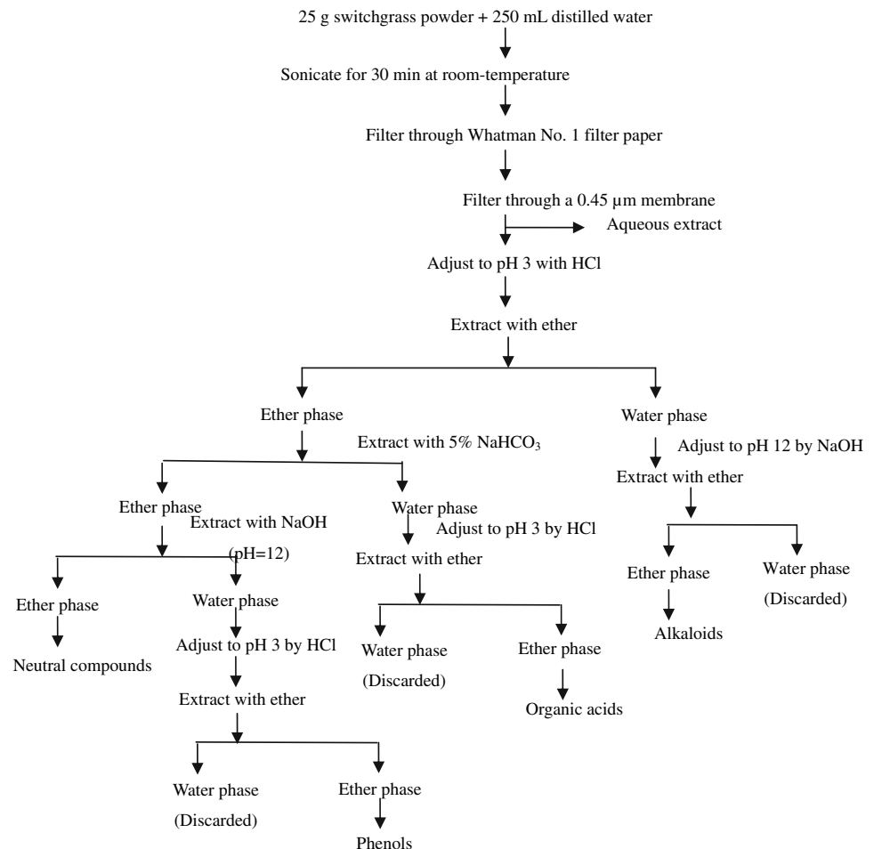
Fig. 1 Extraction procedure for isolating allelochemicals in switchgrass
