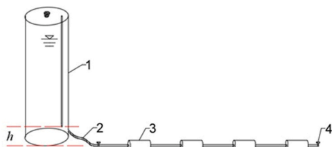
Fig. 2. The hydraulic performance test platform, 1-Mariotte bottle 2- lateral porous ceramic emitter 3- water valve h -working pressure.
