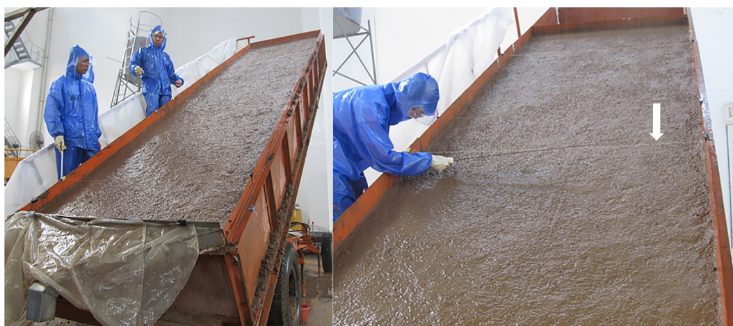
Fig. 1. Experiment flume setup, the three observation sections were separated by the white lines (white arrow).
